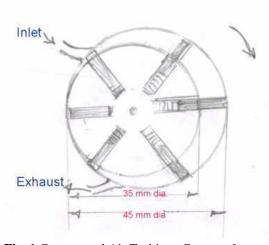
**Fig. 1** Compressed Air Turbine –Concept & Cycle
