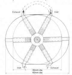
**Fig.5** Dual inlet & exhaust Air Turbine Model
