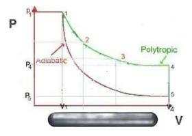
Fig.2 Isentropic cycle for Air Turbine
