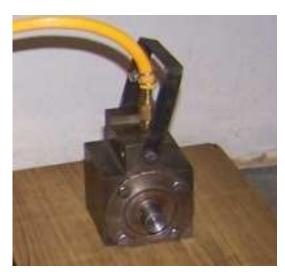
Fig. 3 Compressed Air Turbine-Working Model
