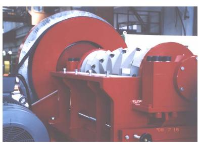
Rough Chopper RC 110 is best suited for the medium throughput cable recycling plant.
