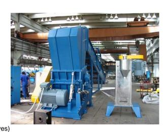
CS Granulator 400#600 (30 kW el. motor, 3 rows of the bed knives and 5 rows of the fly knives) http://share.pacomlan.com/images/yNz31202.pdf Rubber Bales Granulator
