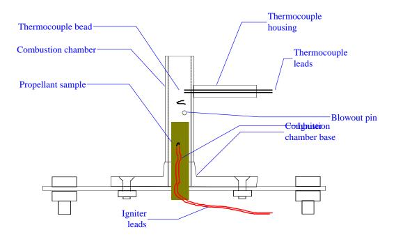
Combustion chamber: 1/2 black iron pipe thread 1/2NPT bottom end Thermocouple: Type C, Tungsten-5% Rhenium vs Tungsten-26% Rhenium Thermocouple housing: 1/8 black iron pipe, threaded 1/8NPT one end with two ceramic insulating tubes epoxied within Results:
