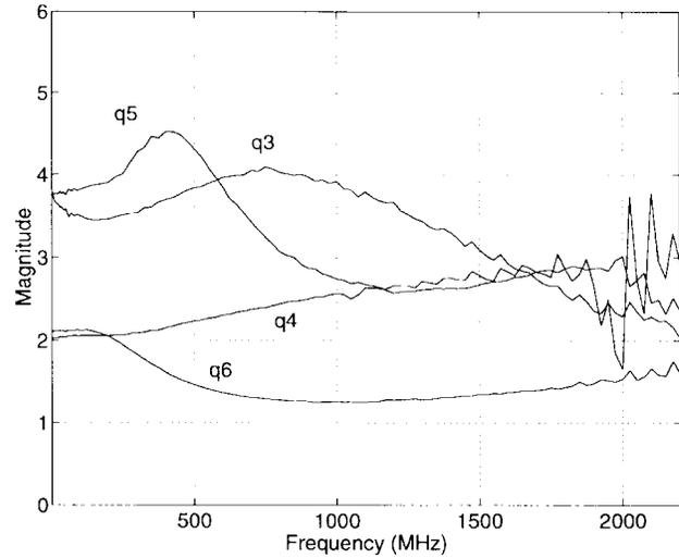
Fig. 4. Magnitudes of the measured  $q$ -points of the six-port reflectometer shown in Fig. 2.
