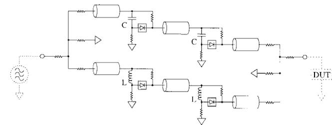
Fig. 2. Schematic of the second new six-port structure (without explicit reference detector).
