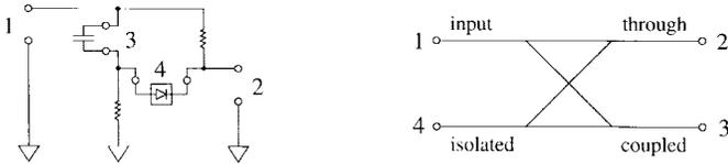
Fig. 3. Schematic of the reflector bridge (left) and the equivalent directional coupler (right).
