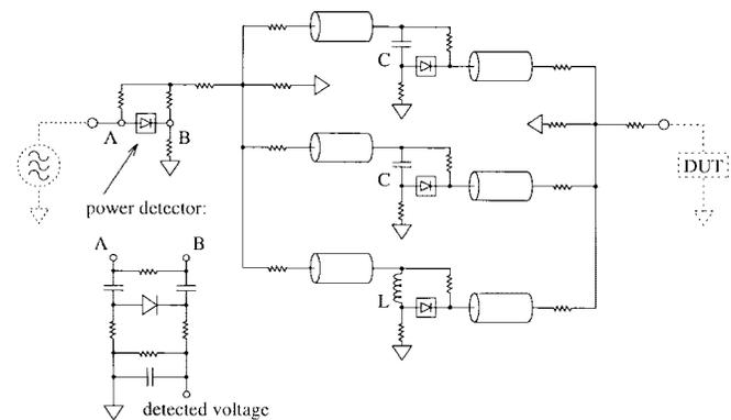
Fig. 1. Schematic of the first new six-port structure (with detailed view of a power detector).
