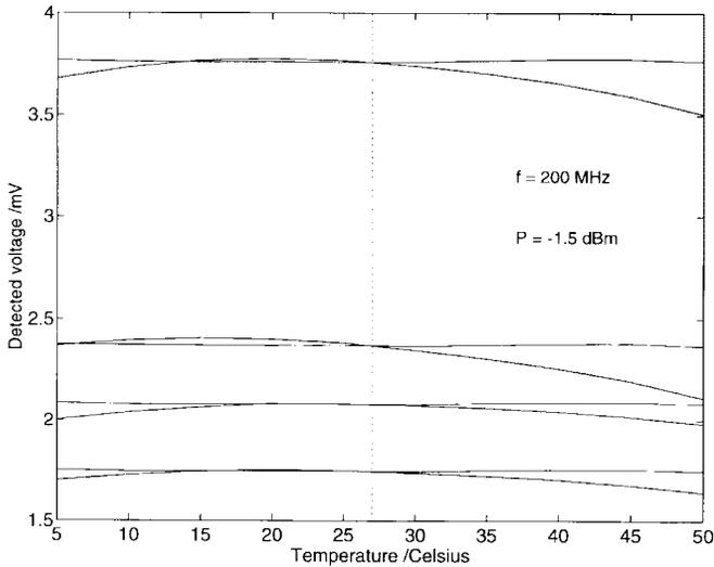
Fig. 6. Detected voltages at the four power detectors as a function of temperature. The almost straight lines represent the corrected values interpolated from the lookup-tables.
