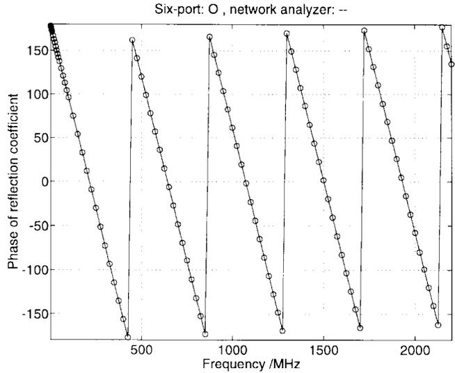
Fig. 7. Phase of the reflection coefficient of a test load, measured with the six-port reflectometer shown in Fig. 2 (circles) and a commercial network analyzer (solid line).
