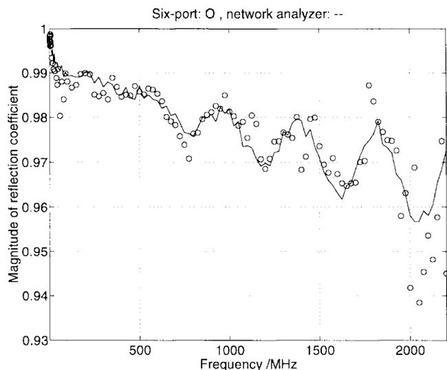
Fig. 8. Magnitude of the reflection coefficient of a test load, measured with the six-port reflectometer shown in Fig. 2 (circles) and a commercial network analyzer (solid line).
