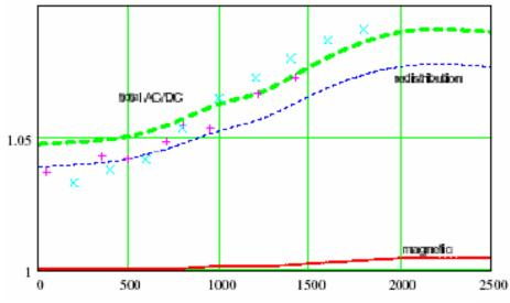
Notice that the core losses and transformer effect (magnetic coupling) is stronger for 3-layers of aluminum strands
