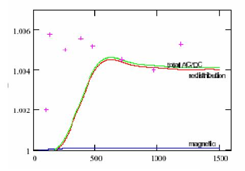
Notice that the core losses and transformer effect (magnetic coupling) is small for 2-layers of aluminum strands
