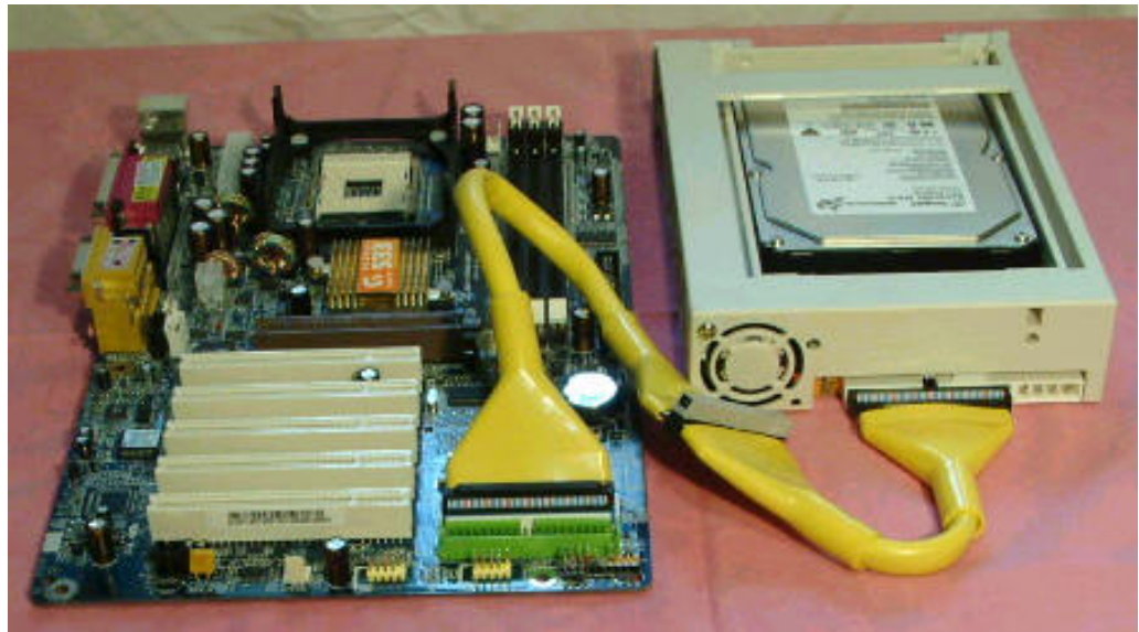
Connecting IDE cable from Mobile Rack to the Mother Board
