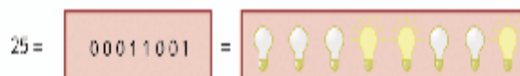
Figure 1-3 All letters and numbers are stored in a computer as a series of bits, each represented in the computer as on or off
