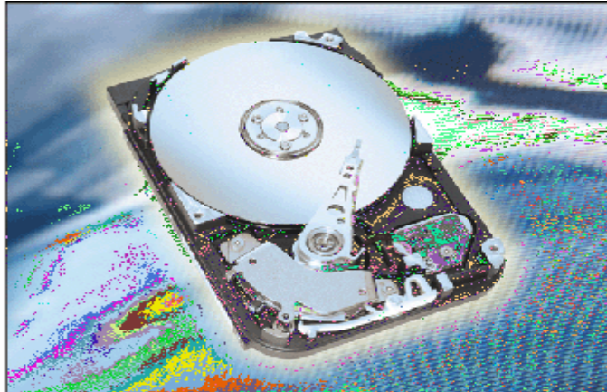
Figure 1-16 Hard drive with sealed cover removed
