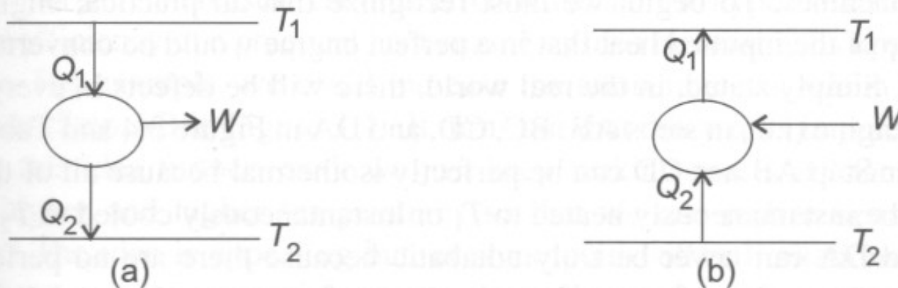
Figure 3.3. Two combinations of continuous heat and work flows between a high temperature ( T_1 ) and a low temperature ( T_2 ) heat reservoir, allowed by the First and Second Laws of Thermodynamics. The ellipse represents a device that can produce work from heat or utilize work to move heat from a lower to a higher temperature. For reversible systems (see text), Case (a) is a Carnot heat engine and Case (b) is a Carnot heat pump. Adapted from Levenspiel (1996).
