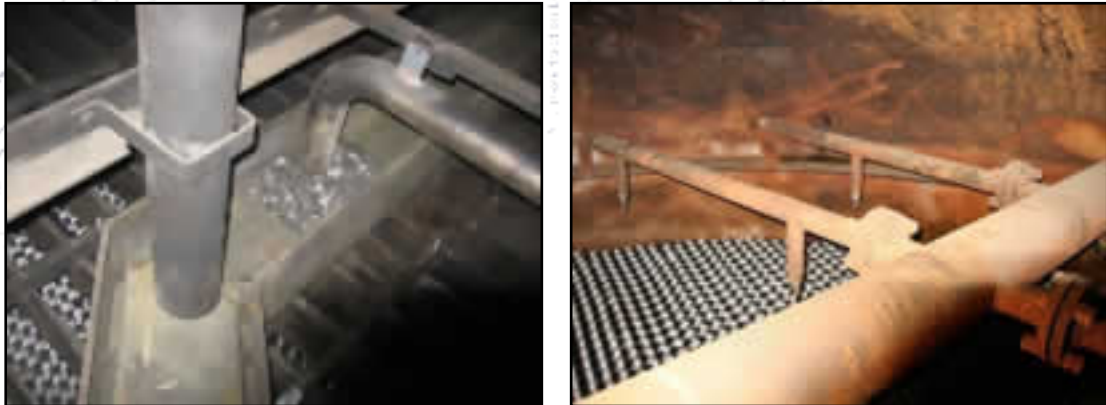
Liquid distributors - Gravity (left), Spray (right) (photos courtesy of Paul Phillips)
