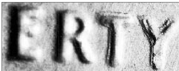
Abrasion doubling shows on the TY of LIBERTY on this 1976 cent, listed elsewhere as a doubled die. Note how the doubling coincides with the area where the clash marks can be seen on the 1970-S cent below.
