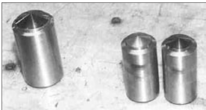
These are blank steel rods used in the hubbing press to get Master Dies, Working Hubs or Working Dies.
