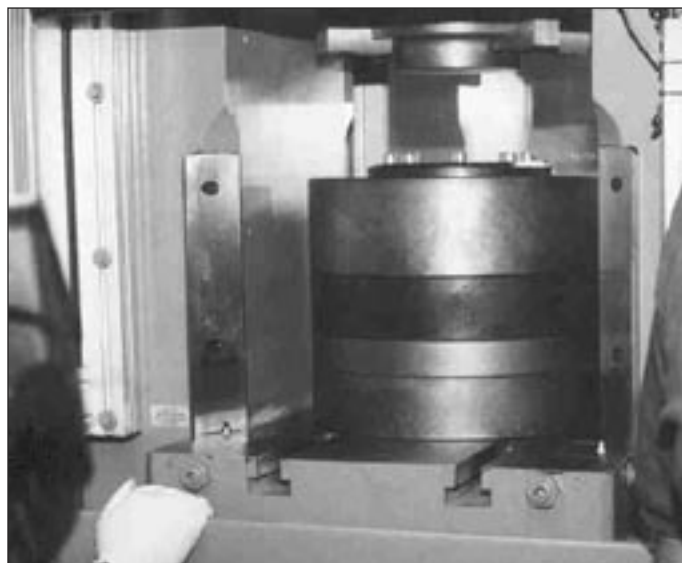
This is one of the hubbing presses in use in the die making shop at the Philadelphia Mint in June of 1998. It is a single-squeeze hubbing press . It allows dies and hubs to be produced with just a single hubbing as opposed to the multiple hubbings that were required in the past.
