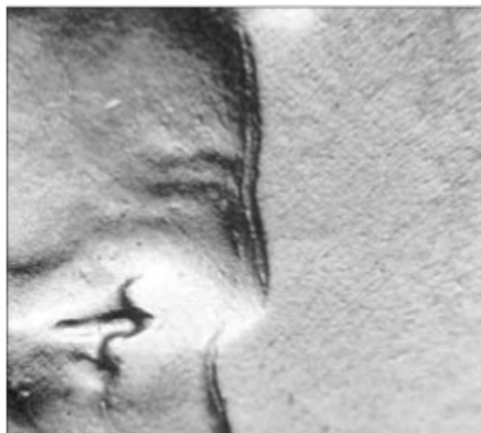
This photo shows the reduction lathe doubling found on Lincoln's forehead on cents dating from the early thirties into the fifties. This doubling adds no extra value to the coins since it is far too common.
