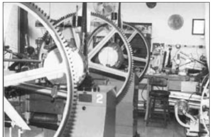
This photo shows several Janvier Reduction Lathes in use at the Philadelphia Mint. This photo was taken during a tour of the Mint that we were a part of in June of 1998. These lathes are used to transfer the design from a twelve to fifteen inch galvano onto the face of a steel bar that will become the Master Hub.
