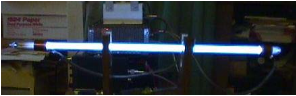
This is the same tube energized, with copper collars as electrodes.
