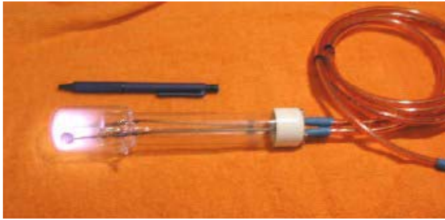
Hand held mini P-tube shown in its energized state.
