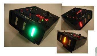
Instead of keeping 3 separate equipment (stopwatch, bell and traffic lights), the T-FIT integrates them all into 1 nifty box. The lights are big and bright, and impossible not to see them. The display and buttons and big enough to operate comfortably. And the machine is light weight and small enough to be taken home or from club to club.
