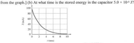
a) According to the figure,  $I_0 \approx 95 \text{ mA}$  and  $\tau \approx 2.5 \text{ ms}$ . At  $t = \tau$ ,  $I = \frac{I_0}{e} = \frac{0.095 \text{ A}}{2.718} = 0.035 \text{ A}$ . Find  $Q_0$ .
