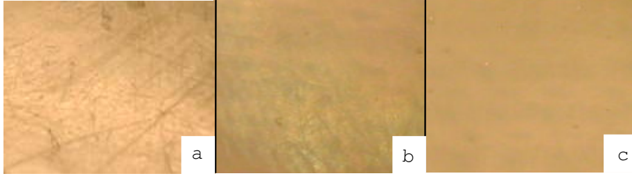
Figure 14: Surface of H_2 -plasma treated FEP. (a) is virgin FEP, (b) is treated with 40 J.mm^{-2} , (c) with 120 J.mm^{-2}
