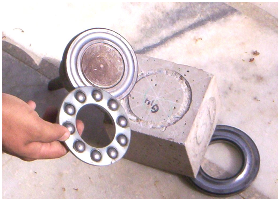
Fig. 4 – Indentation caused by revolving ball ring in the Abrasion test
