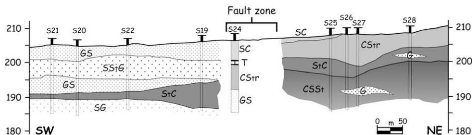
**Fig. 10.** Sketch across the fault zone along the Volturno Valley (trace B in Fig. 7). According to bore-hole stratigraphy, the footwall and hangingwall show two different depositional successions (mainly gravel and sand the former, vs silt and clay the latter). Bore-hole S24 falls in the fault zone, and shows the reddish (r), oxidized silty clays (see CStr in the footwall) lowered by ~10 m. G, gravel; S, sand; St, silt; C, clay; T, travertine.
