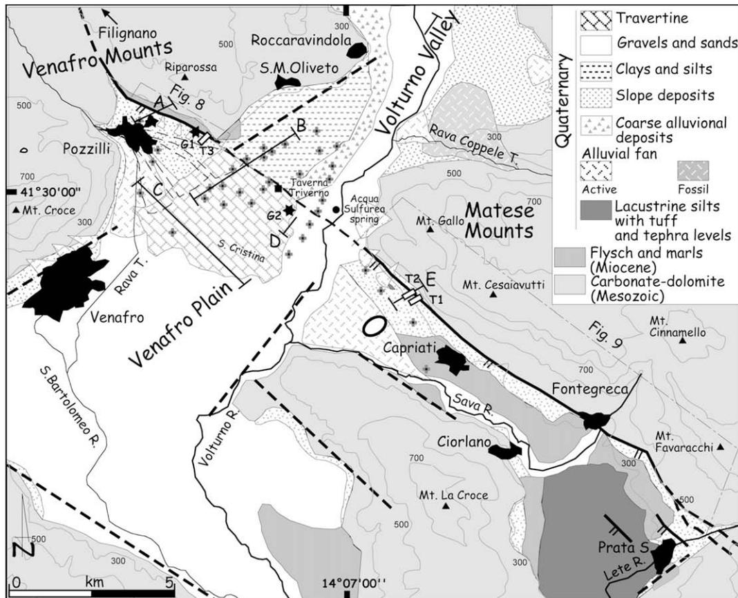
**Fig. 7.** Simplified geological map of the investigated area, based on data from SGN (1971), Corniello et al. (1999), Otterloo van (1981), and on aerial photograph interpretation and field survey. G1 = geomagnetic survey; G2 = electrical resistivity tomography; T1, T2, T3 = paleoseismological trenches; A, B, C, E = traces of geological sketches; D, fluvial terraces profile; cross symbols indicate bore-holes. Bold line is the Aquae Iuliae fault; dashed lines, inferred and/or buried faults.
