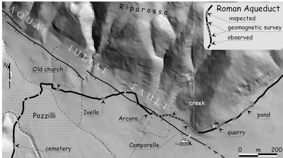
**Fig. 23.** Shaded relief view of the area crossed by the buried Roman aqueduct near Pozzilli (from 1:5,000 maps). Note that the aqueduct is cut by the northern segment of the Aquae Iuliae fault several times between the Ivella and creek sites. A precise topographic levelling of this tract is shown in Fig. 25. The backhoe symbol indicates the site of trench 3.
