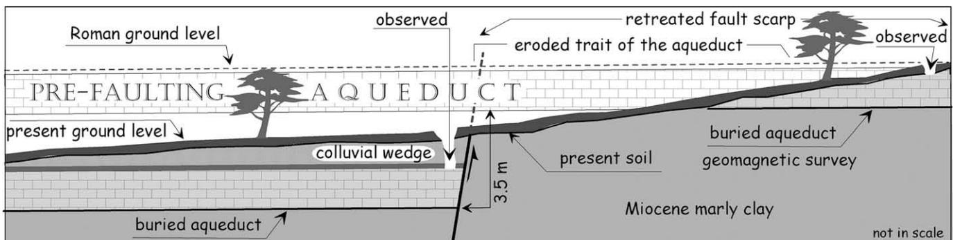
**Fig. 26.** Sketch of the aqueduct in the fault zone (not to scale). Relics of the aqueduct were seen and their altitude was calculated, both in the hangingwall and in the footwall (arrows). Here, the absence of the tunnel nearing the fault has been confirmed by geomagnetic analyses.
