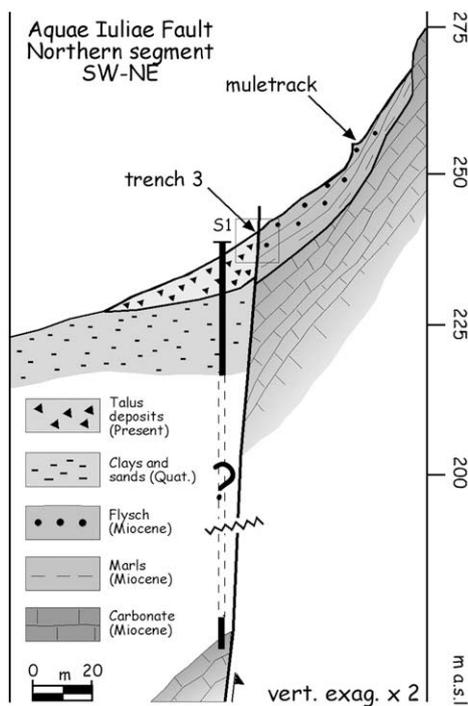
**Fig. 14.** Geological section across the northern segment of the AIF (trace A in Fig. 7). The main scarp along the slope is controlled by the subvertical limestones–marls passage, whereas the fault does not show any prominent morphological evidence. S1, bore-hole reaching the carbonate basement.
