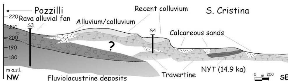
**Fig. 11.** Sketch across the travertine plate (C in Fig. 7), showing the stratigraphical relationships amongst the different Late Pleistocene units of the area (vertical exaggeration × 10). The tephra level has been identified with the Neapolitan Yellow Tuff (~15 ka; see Tab. 3; B. Giaccio, pers. com.). Mod. after Otterloo van (1981), according to bore-hole data, geoelectrical tomography (ERT), and field survey.
