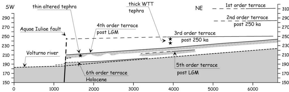
**Fig. 13.** Terraces profile along the left bank of the Volturno River in the investigated area (elevations are from 1:5,000 maps; trace D in Fig. 7). Note the lack of all the terraces in the hangingwall (simple lines are degradational terraces; hatches, depositional terrace). WTT is the Roccamonfina volcano White Trachitic Tuff (see text).
