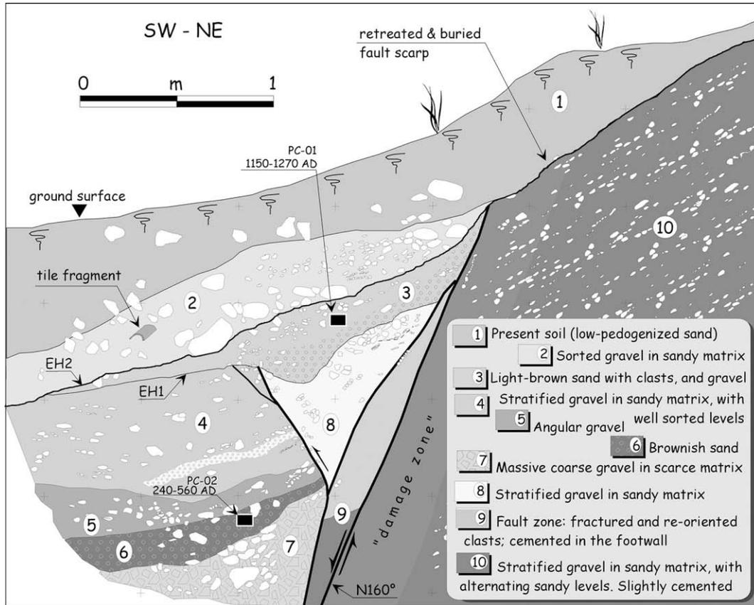
**Fig. 19.** Sketch of the second trench excavated across the AIF, at the foothill of Mount Cesaviutti. The last event occurred after 1150 to 1270 AD, whereas a previous one (or more than one) occurred some time after 240 to 560 AD. Also in this case, the age of the last rupture matches with the 1349 earthquake.
