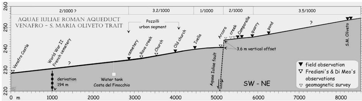
**Fig. 25.** Real altimetric profile of the Roman aqueduct between Venafrò and S. Maria Oliveto. Note the step seen between the two strands (Venafrò–Arcora vs Camporelle–S. Maria Oliveto), which occurs just at the fault crossing point. A continuous deformation, revealed by the lowering of the gradient, occurs as nearing the fault on both sides. For simplicity, this section does not show other possible fault/aqueduct intersections between Arcora and Iviella (e.g., in Fig. 23).
