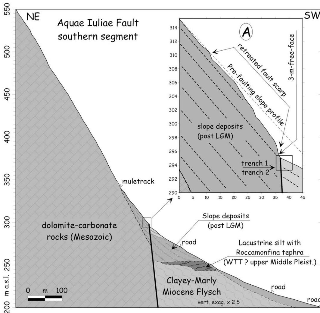
**Fig. 16.** Geological section along the Mount Cesaviutti slope (vertical exaggeration  $\times 2.5$ ; section E in Fig. 7). Trenches 1 and 2 were dug into well-stratified slope gravels, at the base of the fault scarp that interrupts the post-LGM rectilinear slope profile (see inset A).
