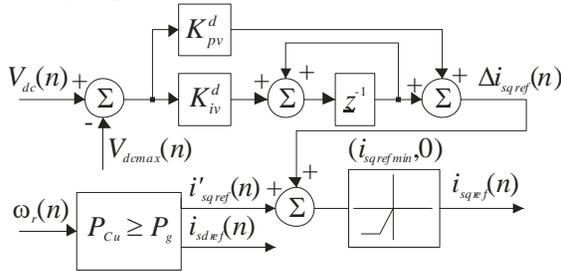
Fig. 2 Block-diagram of braking control system
