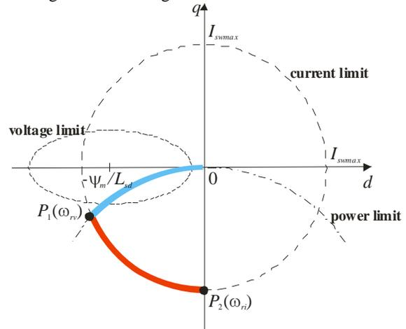
Fig. 1 Trajectory of stator current space vector during braking
