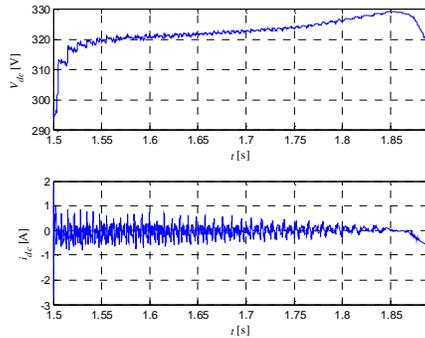
Fig. 5 DC link voltage and current during braking
