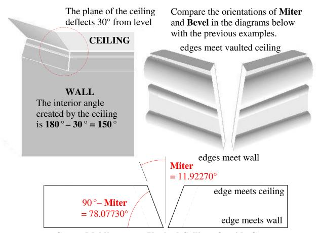
**Crown Molding meets Vaulted Ceiling: Outside Corner** The saw blade angle or **Bevel** is oriented to make the visible face of the molding longer than the face toward the wall.
