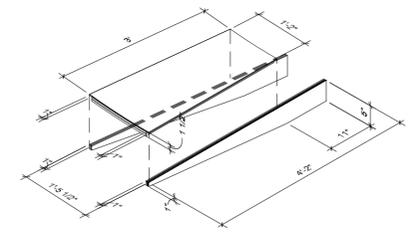
Exploded Axonometric of Tread and Riser
