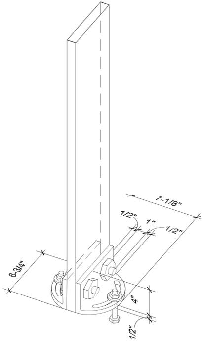
Axonometric of Metal Floor Connection
