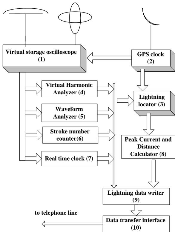
Fig.2. Lightning data acquisition algorithm.
