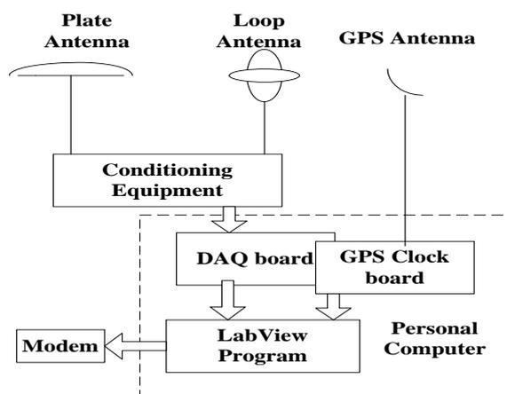
**Fig.1. Block-diagram of lightning detecting and locating station.**
