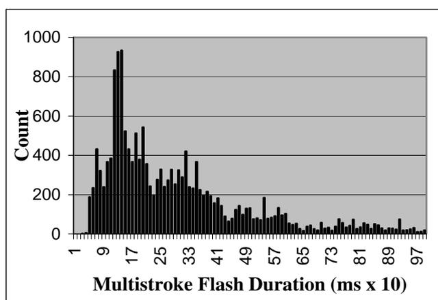
**Fig.3. Multi-stroke flash duration distribution (stroke order 2-12).**
