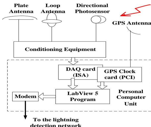
**Fig.1. Block-diagram of Advanced Lightning Detecting and Locating Station.**
