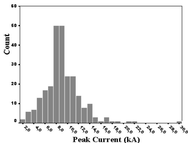
Fig.7. "Isolated pulse" peak current distribution.
