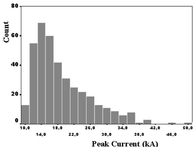
Fig.5. Negative stroke peak current distribution
