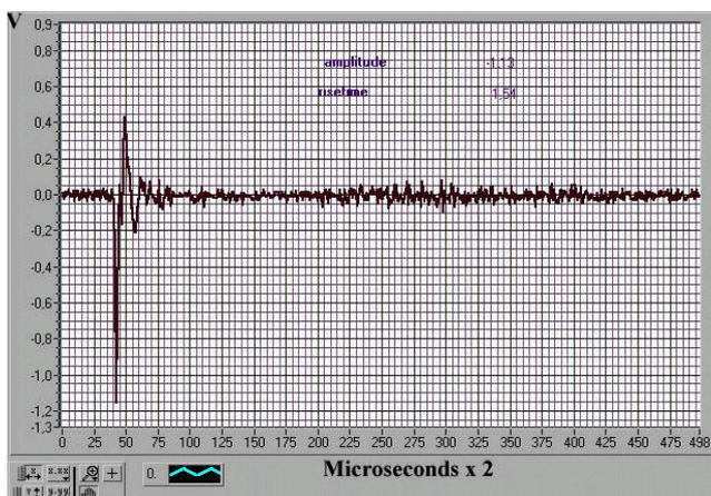
Fig.6. Typical isolated pulse waveform.
