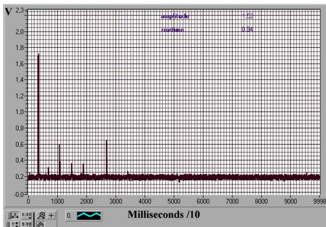
**Fig.2. Six-stroke ground lightning registered by photosensor.**
