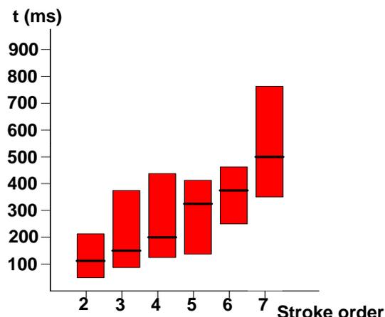
**Fig.4. Lightning flashes duration vs. stroke order.**
