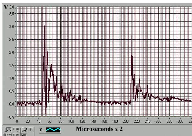
Fig.8. Typical twin-peak ground negative stroke.
