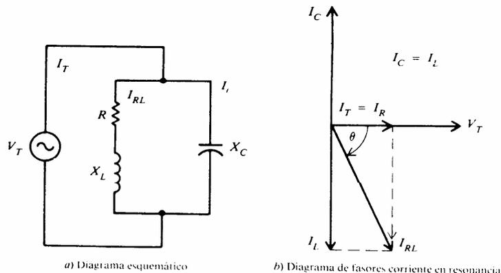
Fig. 4 Circuito paralelo real LC
