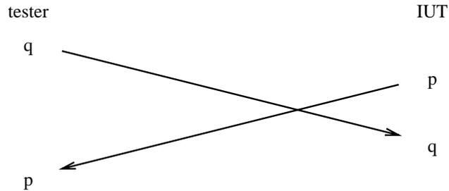
Figure 1.2: Different sequences of events at the tester and at the IUT
