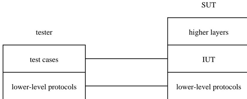
Figure 1.1: The basic conformance testing architecture
