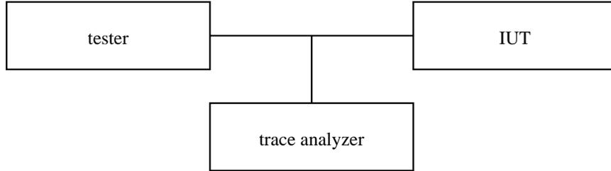
Figure 1.3: Using a trace analyzer for conformance testing
