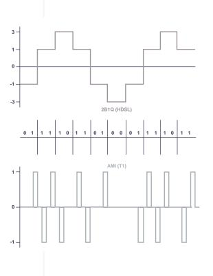
This process is repeated when transmitting from the customer to the network. Upon receiving the standard T1 from the customer premises, the HTU-R completes the same conversion process. Both HDSL signals are encoded with a 2B1Q format and transmitted on both loops.
