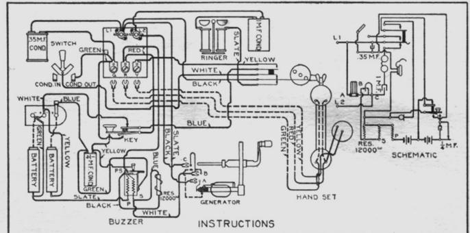
THIS TELEPHONE IS INTENDED FOR UNIVERSAL USE IN CONNECTION WITH TELEPHONE, BOTH MAGNETO AND COMMON BATTERY, TELEGRAPH AND BUZZER LINES. THE SMALL KNFE SWITCH SHOULD REMAIN CLOSED AT ALL TIMES EXCEPT WHEN TELEPHONE IS USED ON TELEGRAPH OR SIMILAR LINE WHERE IT IS UNDESIRABLE TO SHUNT THE LINE BATTERY CURRENT. TO USE AS A COMMON BATTERY TELEPHONE, REMOVE HAND SET FROM HOOK AND CALL SWITCHBOARD IN USUAL WAY. UNLESS KNIFE SWITCH IS CLOSED, SWITCHBOARD OPERATOR CAN BE HEARD BUT CANNOT BE CALLED.
