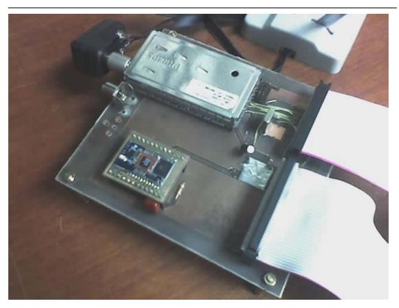
**Fig 10.** The bluetooth TV tuner daughtercard, showing the bluetooth module and TV tuner FOD1216, and the connection to antenna.
