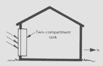
Buckley tank installed in south wall of house. Vertical cross section, looking west.
