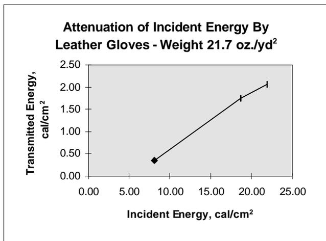
about 40% of the incident energy. Adding the polycarbonate faceshield further reduced the eye and
