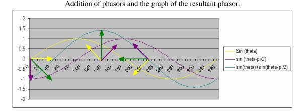
The instantaneous power of the circuit is  $P(t) = V_T(t) I(t)$ Substituting for  $V_T(t)$  and I(t)  $P(t) = V_{To} \sin (\omega t - \phi) I_o \sin (\omega t)$   $P(t) = V_{To} I_o \sin (\omega t - \phi) \sin (\omega t)$   $P(t) = V_{To} I_o [(\sin \omega t \cos \phi - \cos \omega t \sin \phi) \sin \omega t]$  $P(t) = V_{To} I_o [(\sin \omega t \sin \omega t \cos \phi - \cos \omega t \sin \omega t \sin \phi)]$
