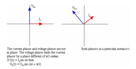
Using Ohm's Law, we have V = IR, then  $V_L(t) = I_o X_L \sin(\omega t + \phi + \pi/2)$ , where  $V_{Lo} = I_o X_L$ .
