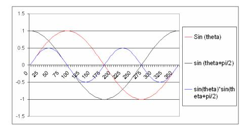
The average power is  $\langle P \rangle = 0$ . Notice in the graph above that there is positive power and negative power. Thus energy is stored in the capacitor and then returned to the circuit.
