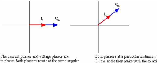
speed  $\omega$ . If  $I(t) = I_o \sin \omega t$  then  $V_r(t) = V_{ro} \sin \omega t$ In the above diagram both are on the x-axis,  $\theta = 0$
