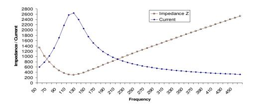
The shape of the current curve becomes sharper if resistance is lower. The "spread" of the hump can be designed to obtain a balance between maximum current and the ability to tune in to the resonance frequency.
