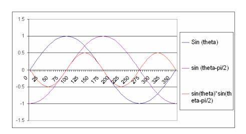
The average power is  $\langle P \rangle = 0$ . Notice in the graph above that there is positive power and negative power. Thus energy is stored in the capacitor and then returned to the circuit.
