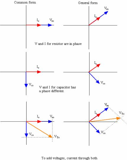
To add voltages, current through both R and C must be of same phase. Current phasor must be aligned for both R and C. Resultant voltage is obtained by vector addition.
