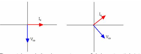
The current phasor and voltage phasor are not in phase. The current phasor leads the voltage pasor by a phase different of  $\pi/2$  radian. If  $I(t) = I_o \sin \omega t$  then
