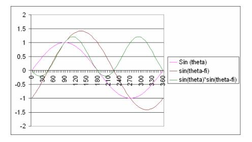
Notice that there is negative power which is the energy returned by the capacitor to the circuit.
