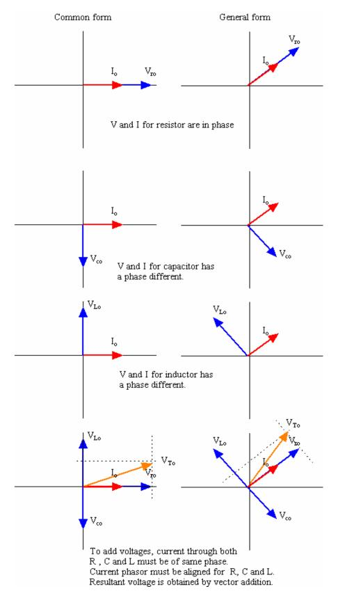
The magnitude of the resultant phasor V<sub>To</sub> can be obtain from Phytagorean Theorem;  $V_{To}^2 = V_{ro}^2 + (V_{Lo} - V_{co})^2$   $V_{To} = \sqrt{V_{ro}^2 + (V_{Lo} - V_{co})^2}$ And the angle between V<sub>To</sub> and I<sub>o</sub> is  $\phi = \tan^{-1} \frac{V_{Lo} - V_{co}}{V}$ , where  $\phi$  can be a positive or negative value.
