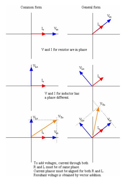
The voltage phasors of the resistor and the inductor are exactly at right angle to each other. The magnitude of the resultant phasor  $V_{To}$  can be obtain from Phytagorean Theorem;
