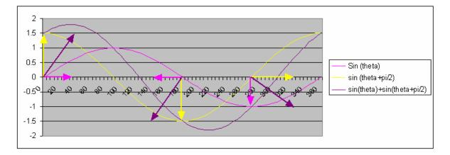
The instantaneous power of the circuit is  $P(t) = V_T(t) I(t)$ Substituting for  $V_T(t)$  and I(t)  $P(t) = V_{To} \sin (\omega t + \phi) I_o \sin (\omega t)$   $P(t) = V_{To} I_o \sin (\omega t + \phi) \sin (\omega t)$   $P(t) = V_{To} I_o [(\sin \omega t \cos \phi + \cos \omega t \sin \phi) \sin \omega t]$  $P(t) = V_{To} I_o [(\sin \omega t \sin \omega t \cos \phi + \cos \omega t \sin \omega t \sin \phi)]$
