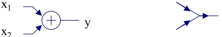
A block diagram element consisting of a circle with a plus sign (+). Two input signals,  $x_1$  and  $x_2$ , enter from the left and converge into the circle. An output signal  $y$  exits from the right. A horizontal arrow points to the right above the output  $y$ .
