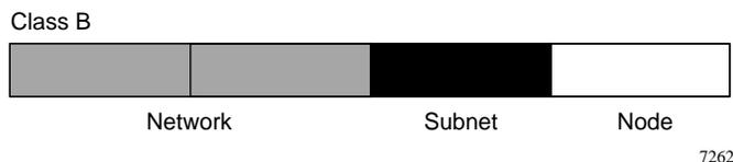
**Figure 10-2. Example of Subnetting a Class B Address**
