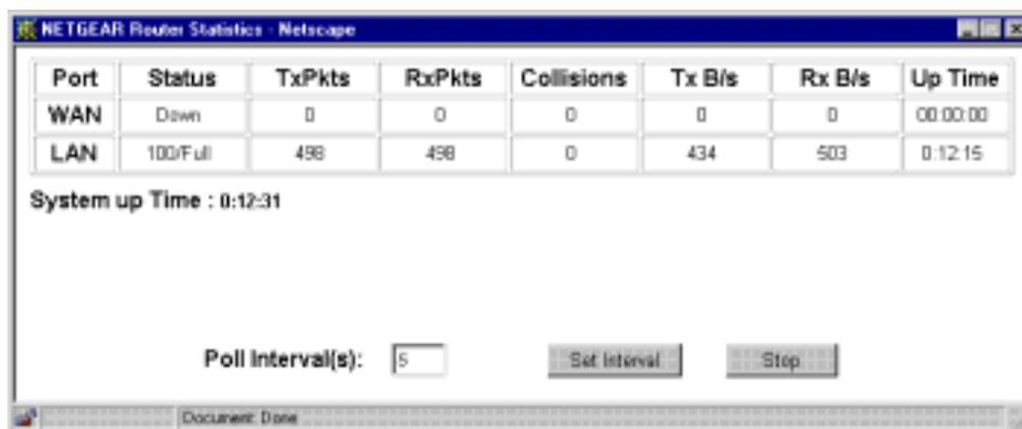
**Figure 4-6. Browser-based configuration, Router Statistics screen**
