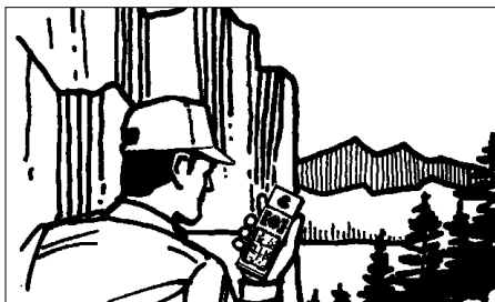
Obstructed View of the Sky
