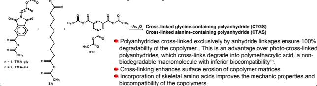
• Polyanhydrides cross-linked exclusively by anhydride linkages ensure 100% degradability of the copolymer. This is an advantage over photo-cross-linked poly(ethylene terephthalate).
