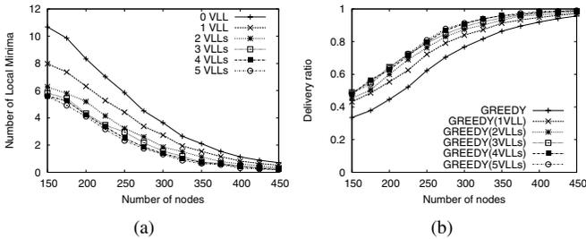
Fig. 1. Effectiveness of the virtual long links in reducing the number of local minima. 2 VLLs means 2 virtual long links per node (a) & Delivery ratio in pure greedy routing protocol (b).
