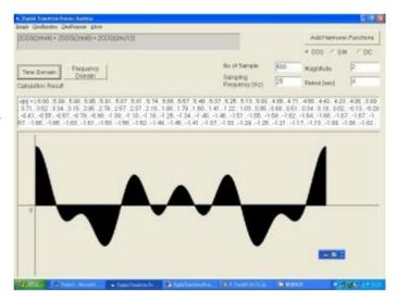
*FileName: DigitalTransformFourierAnalysis.doc* The frequency domain spectrum. Because the number of samples is 600 in this case, the repetition cycle in frequency domain is also 600.
