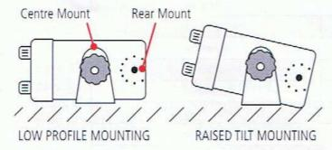
The TX2700 mounting bracket is designed with a unique dual position gimbal mounting slot. This design not only allows the TX4400 to be tilted over a much greater range, but also provides a slim, low profile mounting position for installations where space is very limited.
