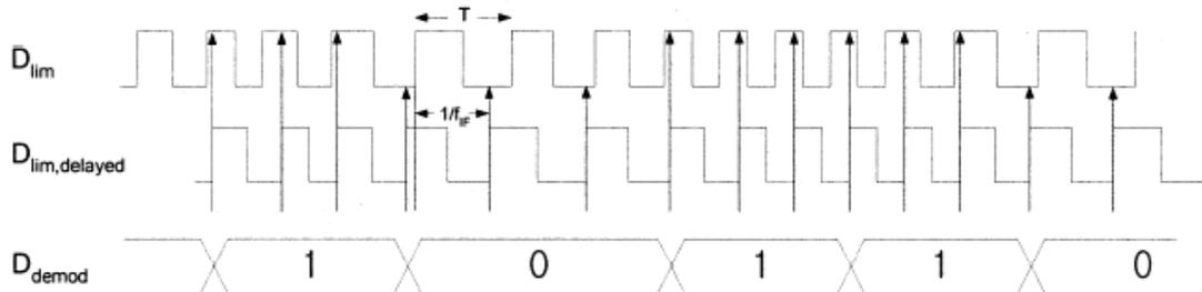
Figure 7.9 Demodulation waveforms
