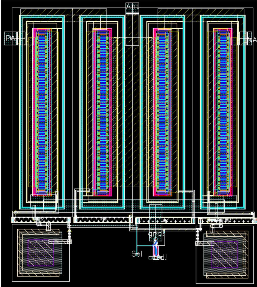
Figure 3.7 Layout of Switch
