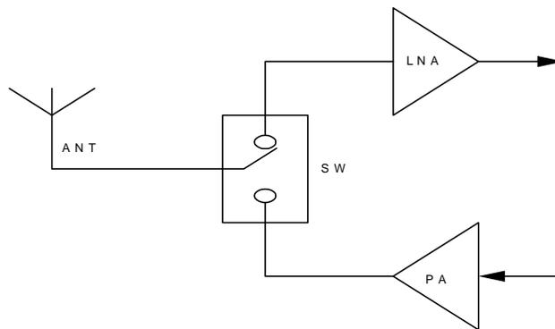
Figure 3.1 Application T/R Switch
