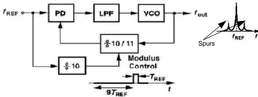
Figure 10.3 Fractional-N Synthesizer
