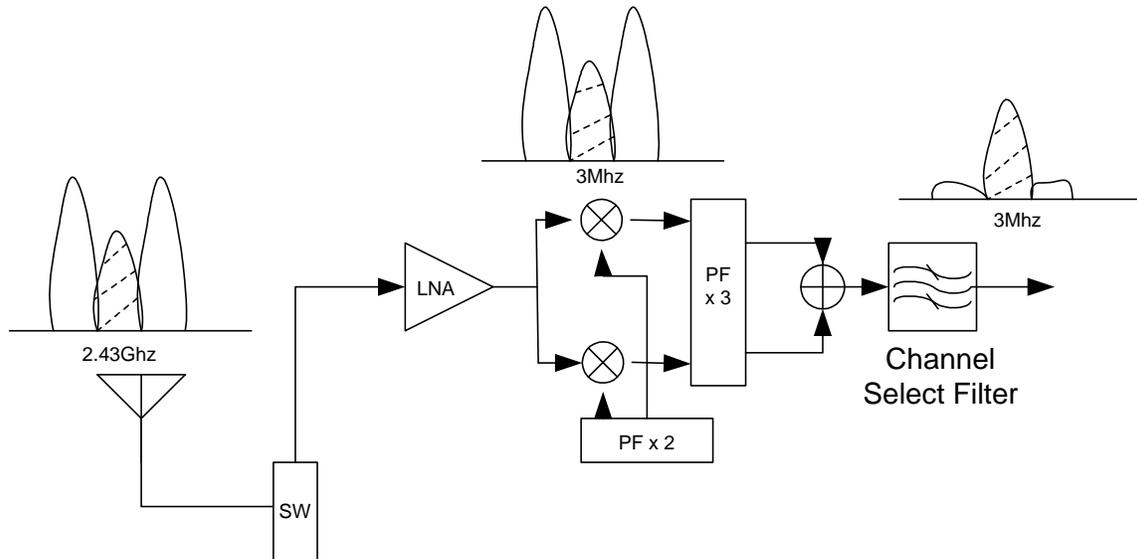
Figure 6.1 Why Channel Select filter is needed in transceiver
