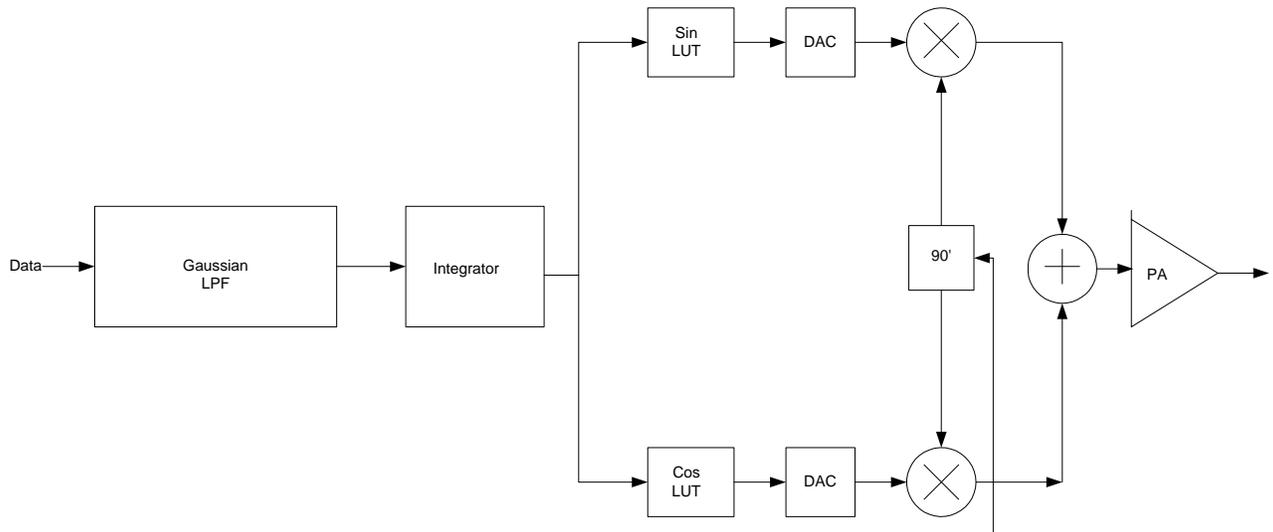
Figure 7.2 Quadrature GFSK Modulations
