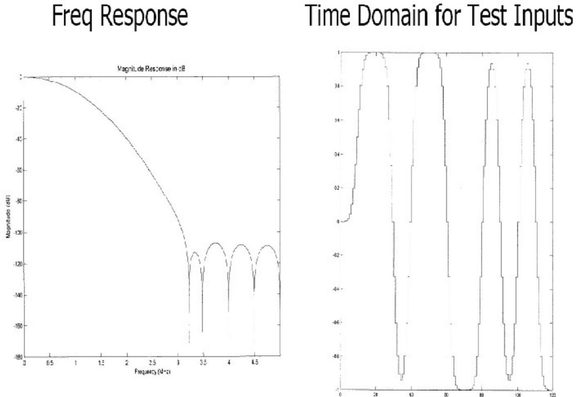
Figure 7.2 Frequency and Transient response of Gaussian Filter
