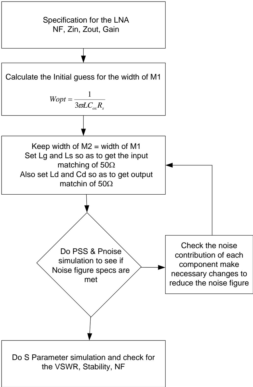
Figure 4-3 Design flow of LNA design
