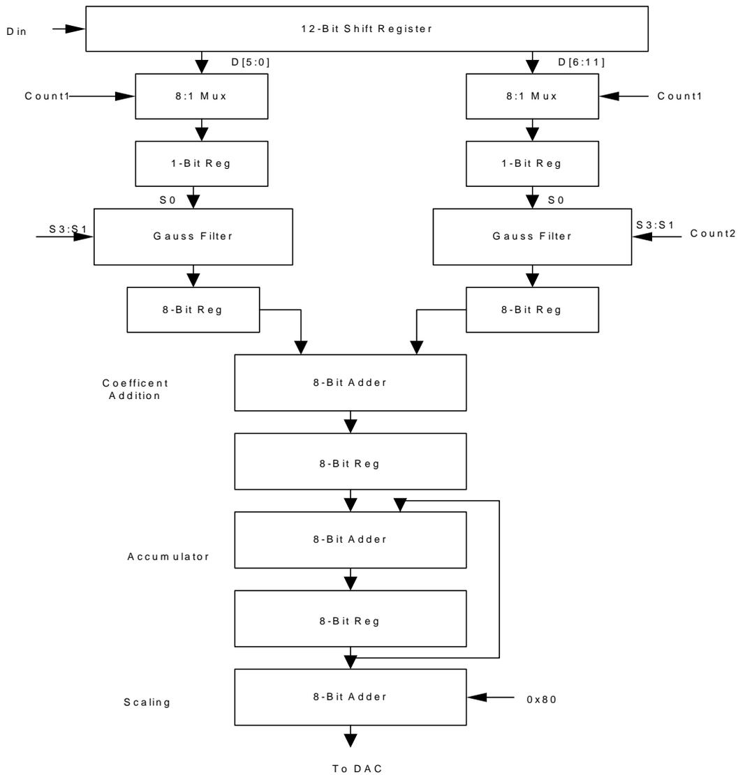
Figure 7.4 Block Diagram of Digital Gaussian Filter
