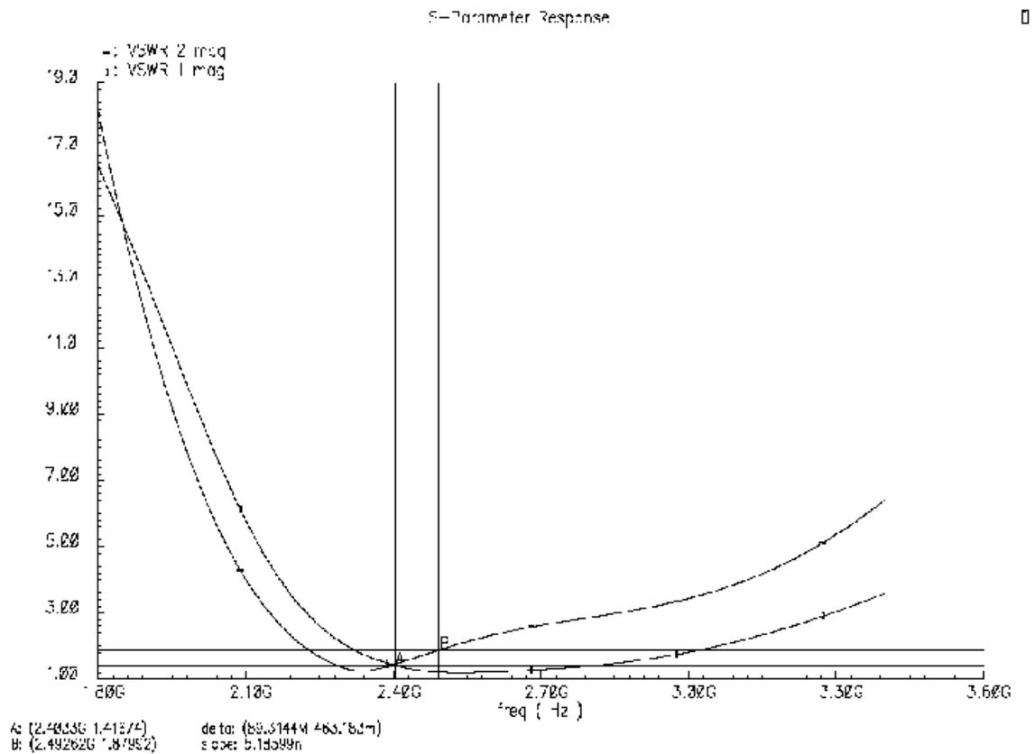
Figure 4.4 Input and Output VSWR of LNA
