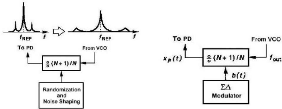
Figure 10.4 A Method for reducing the fractional spurs
