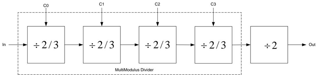
Figure 10.11 MultiModulus divider
