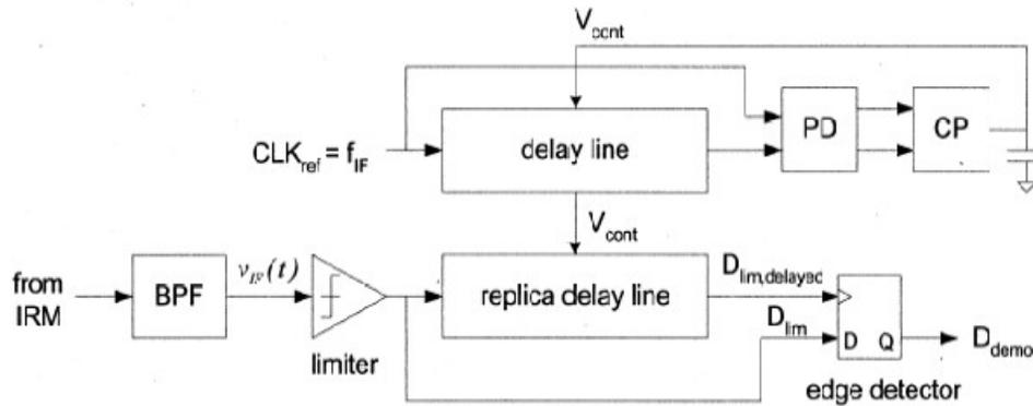
Figure 7.8 DLL based Demodulator
