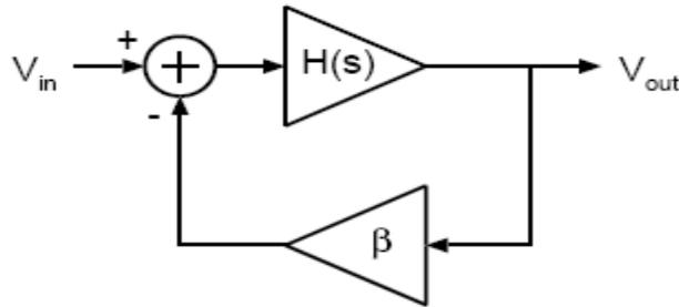
$$\frac{V_{out}}{V_{in}}(s) = \frac{H(s)}{1 + \beta H(s)}$$
