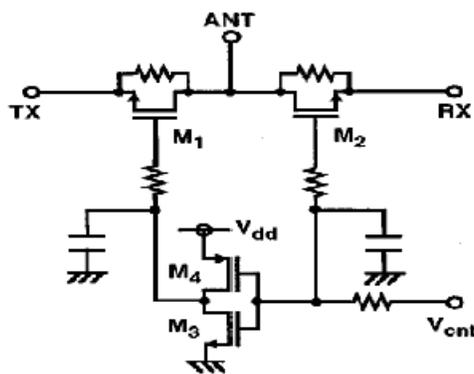
Figure 3.2 Series type Switch
