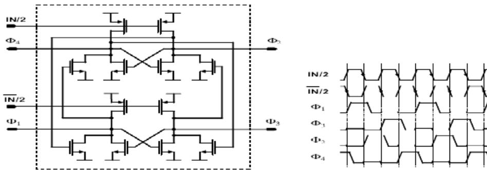
Figure 10.13 Divide by 2 Circuit
