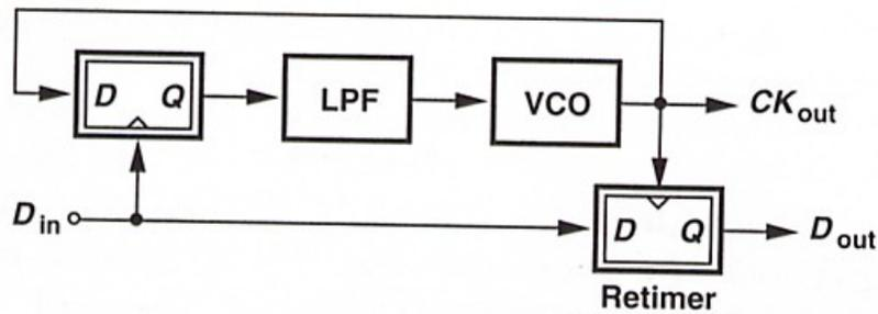
**Figure 8.4 Block Diagram of Clock and Data Recovery Circuit**
