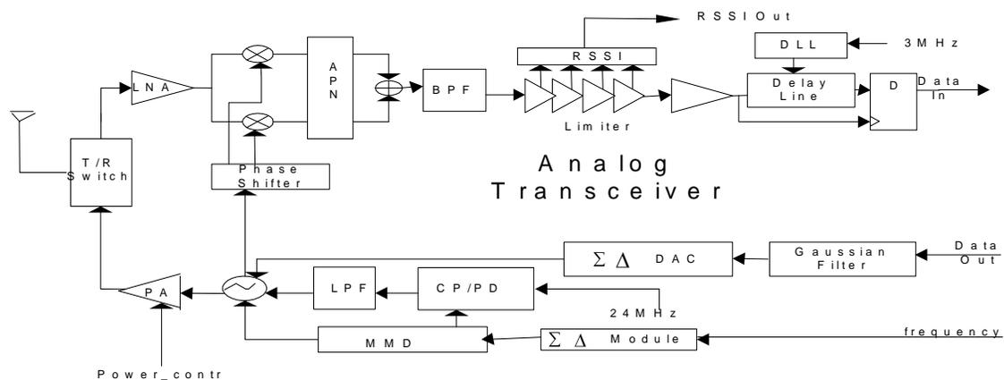
Figure 2.2 Block Diagram of Analog Transceiver
