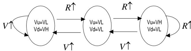
Figure 10.15 Phase Frequency Detector (PFD)
