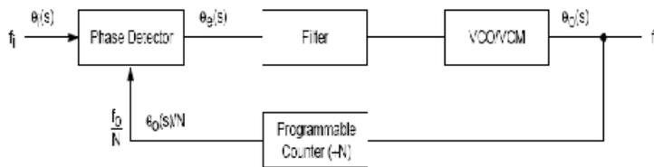
Figure 10.1 Phase Locked Loop
