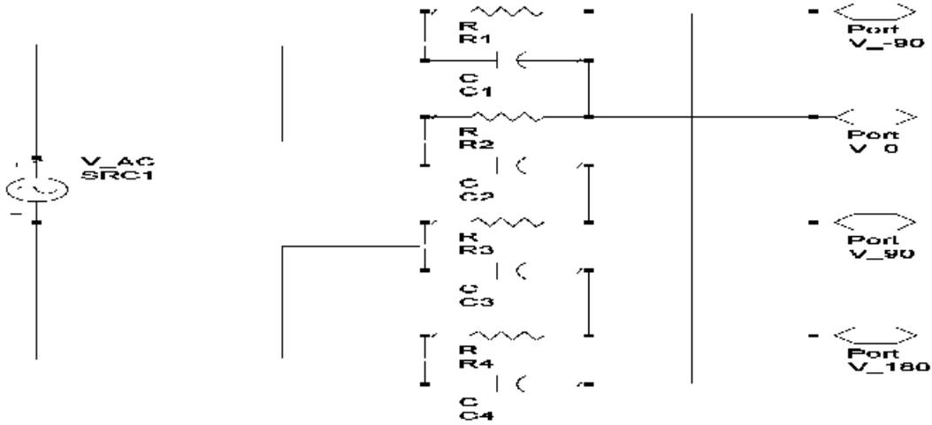
**Figure 5.6 Polyphase filter configured as Phase shifter**
