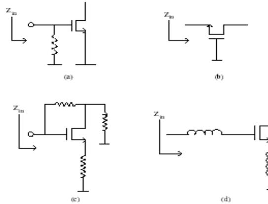
Figure 4.1 Common LNA architectures. (a) Resistive termination, (b)  $1/g_m$  termination, (c) shunt-series feedback, (d) inductive degeneration
