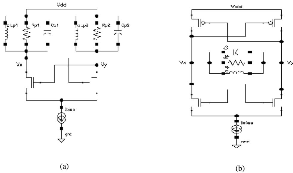
Figure 10.7 (a) Nmos only LC oscillator (b) Nmos-Pmos cross coupled oscillator structure
