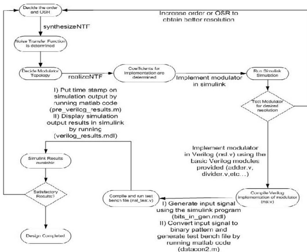
Figure 9.3 Design flow of Sigma Delta D/A converter
