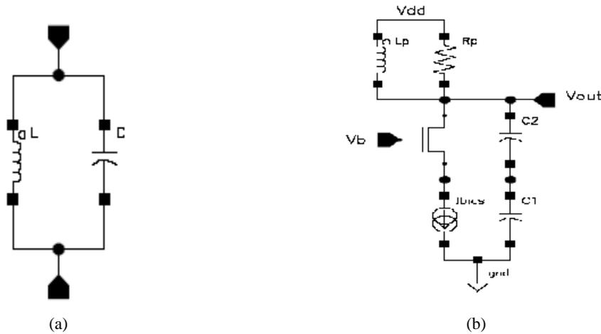
Figure 10.6 a) LC oscillator (b) Colpitts' Oscillator
