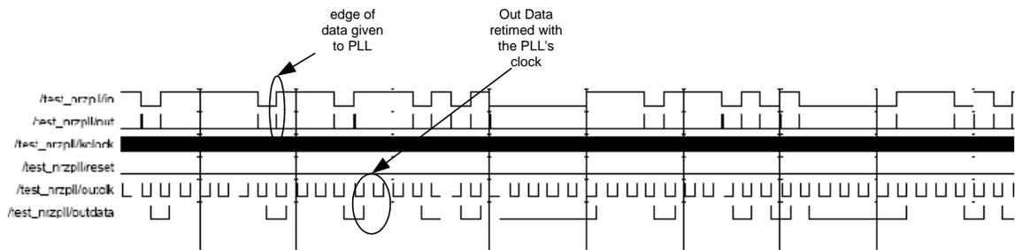
Figure 8.7 Simulation of verilog module of CDR
