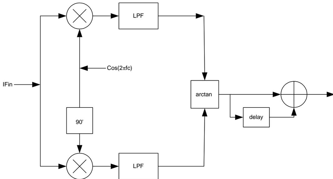
Figure 7.7 Phase Discriminator based gfsk demodulator
