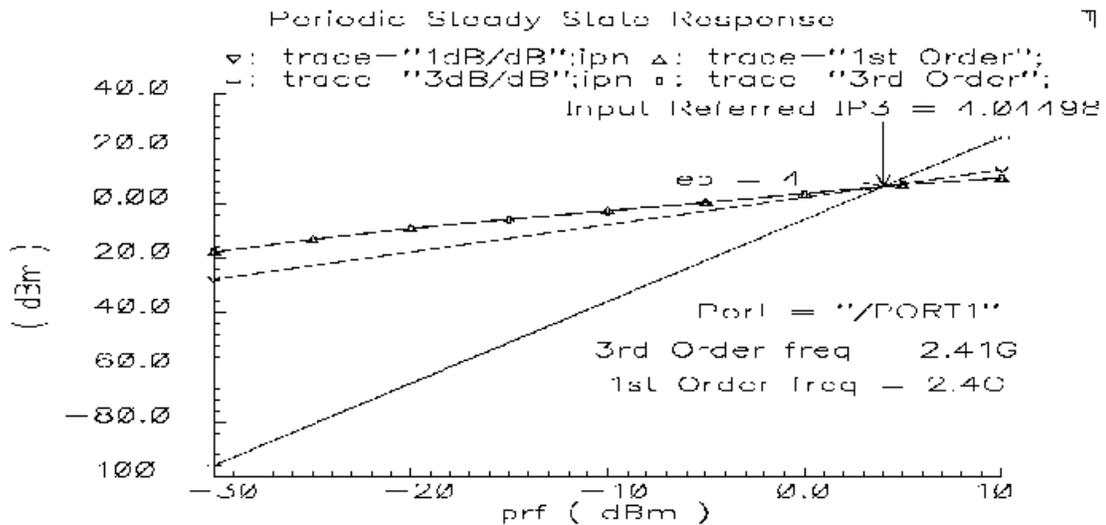
Figure 4.8 IP3 measurement of the LNA design
