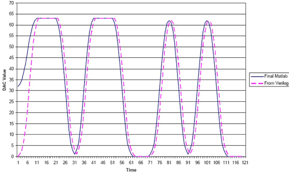
Figure 7.5 Comparison between Verilog and Matlab implementation of Gaussian Filter
