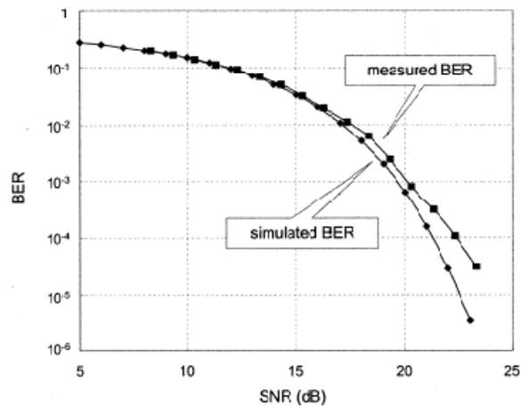
Figure 2.3 BER measurement for DLL based Demodulator [12]
