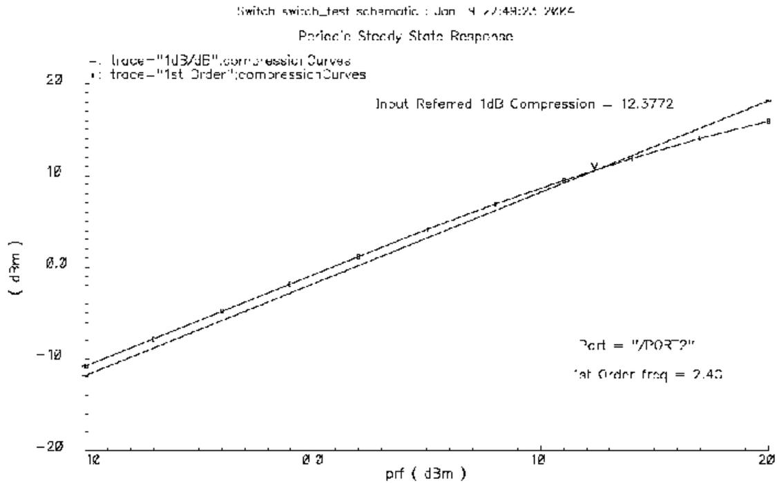
Figure 3.6 1dB compression point of the Switch
