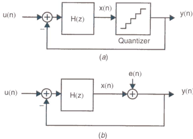
Figure 9.1 (a) First order Sigma Delta Modulator (b) Linear model of the modulator
