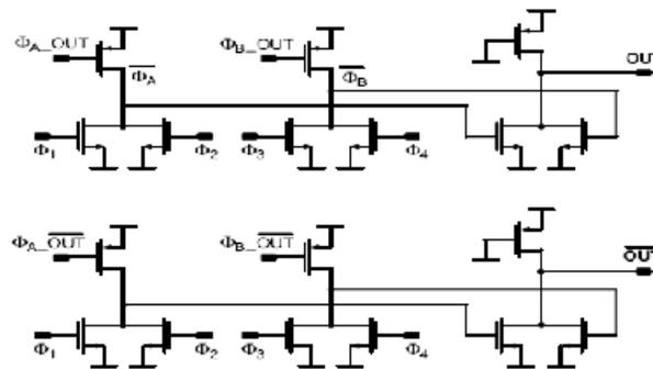
Figure 10.14 High Speed Mux design
