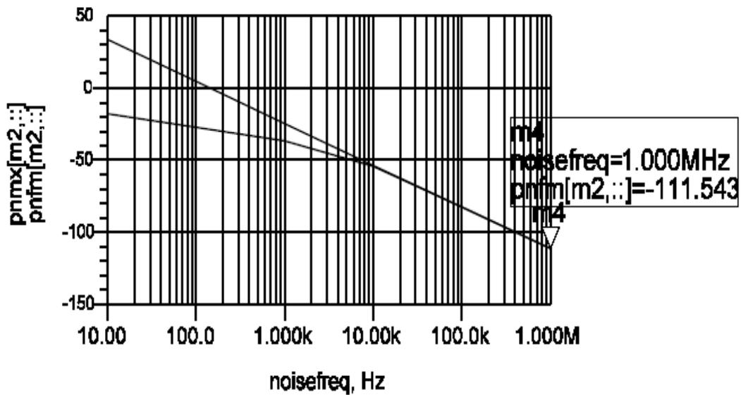
Figure 10.8 Phase noise of the Oscillator
