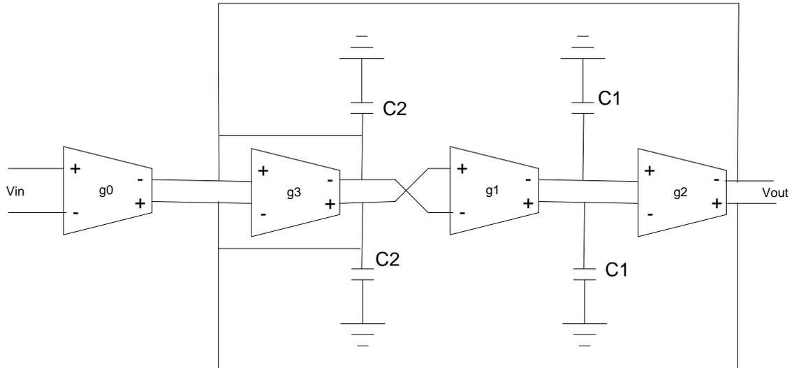
Figure 6.6 Balance structure of Thomas-Tow bandpass OTA-C filter
