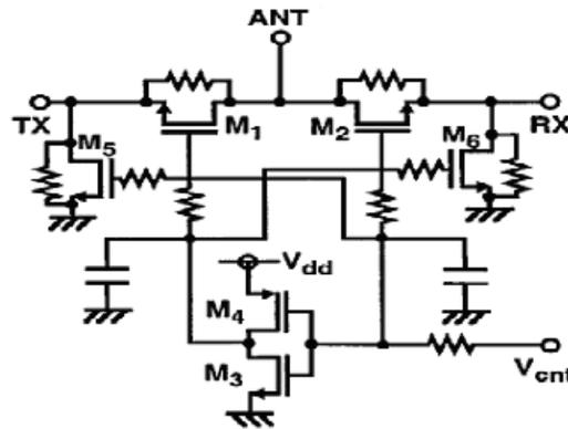
**Figure 3.3 Series/Shunt type Switch**
