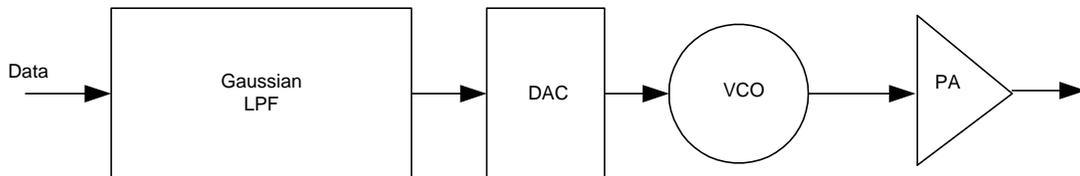
Figure 7.1 Direct GFSK modulations with VCO
