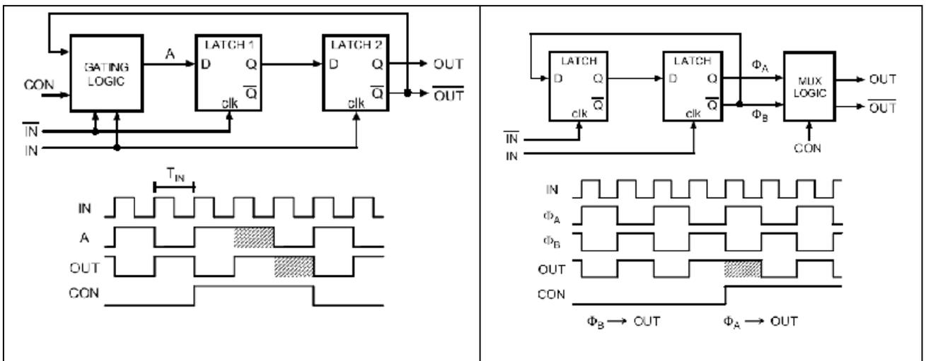
Figure 10.12 Two ways of designing divide by 2/3 circuit
