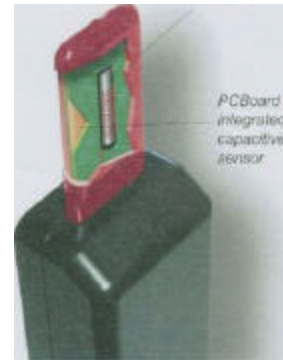
Close up of the PDS sensor
