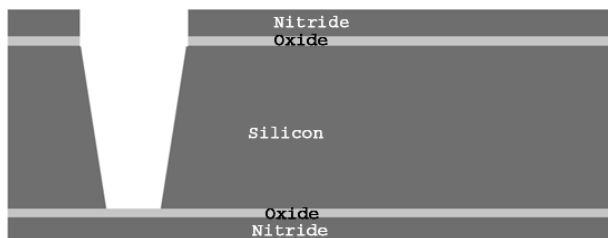
Figure 4. Entry port in top substrate processing.
