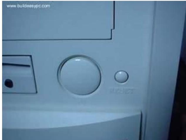
Figure 1 - Power and Reset switch
