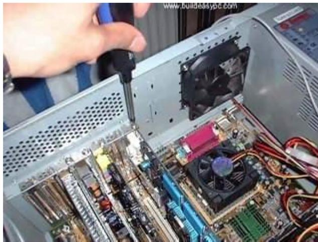
Most modern sound cards are designed with the PCI interface and connect to the PCI slot of your motherboard. A PCI slot looks like the slots on the following image.
