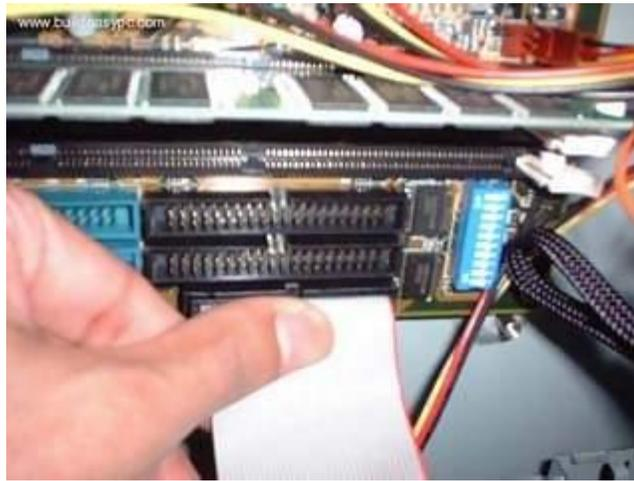
Finally connect the other end of the floppy drive cable to floppy drive connector on your motherboard. Make sure pin 1 on the cable connects to pin 1 on the connector.
