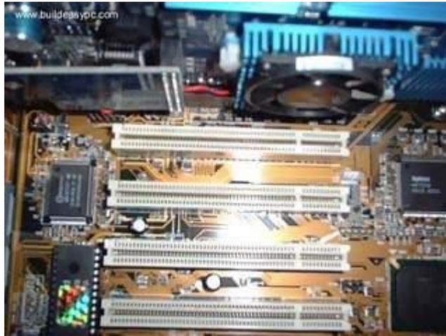
Place your sound card on top of a chosen slot. Gently push down the card so it sits into position. Once the card is seated correctly into position, screw the card on to the case.
