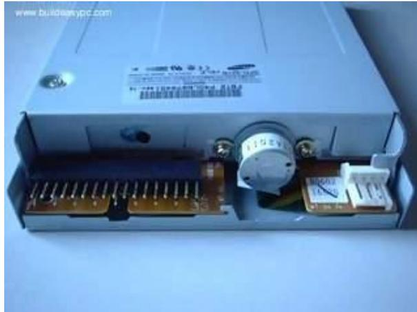
The black connector on the left hand side is the floppy disk connector. It is different from the IDE connector and uses a different cable. The small white connector on the right hand side is the power connector for the floppy drive. Figure 1 and 2 below shows what a floppy drive cable and floppy drive power connector looks like.
