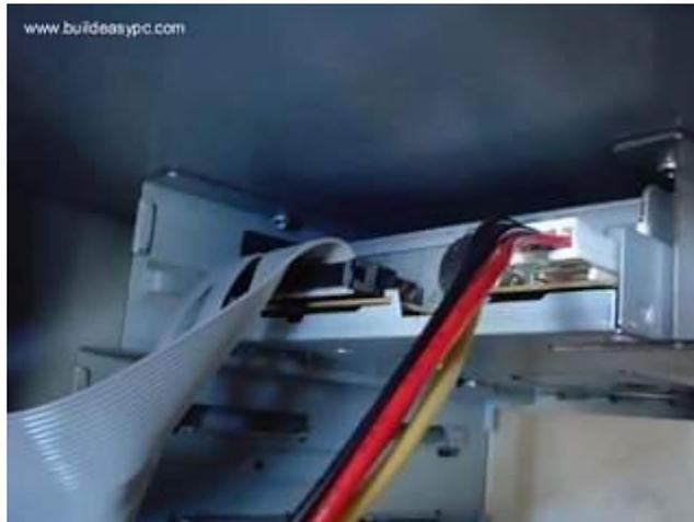
Push the floppy drive power cable to the power connector. This will only go in on way.
