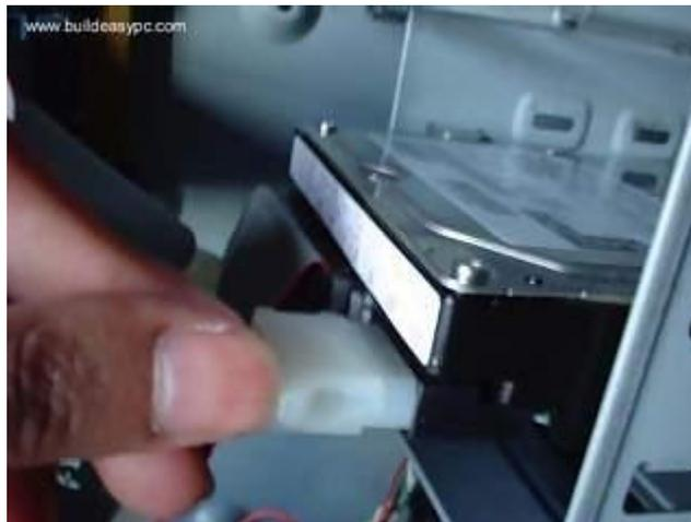
Connect the other end of the ATA 66 cable to the primary ATA socket of your motherboard as shown. Make sure the pin 1 on the cable connects to the pin 1 on the ATA socket.
