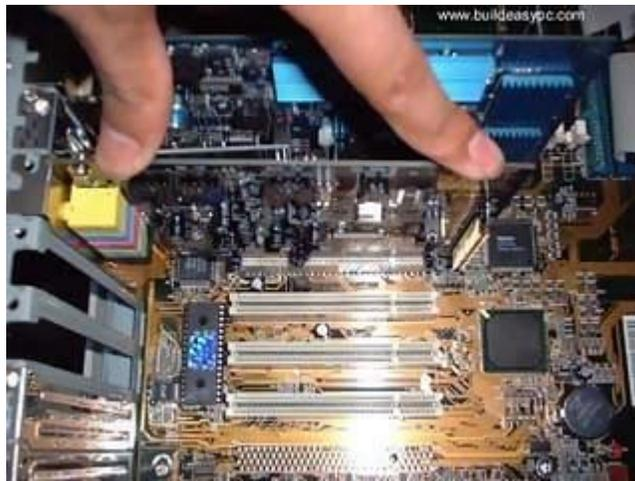
Finally insert the audio cable into the CD-IN socket. The other end of the cable should be connected to Audio-out socket on your CD/DVD-ROM drive.
