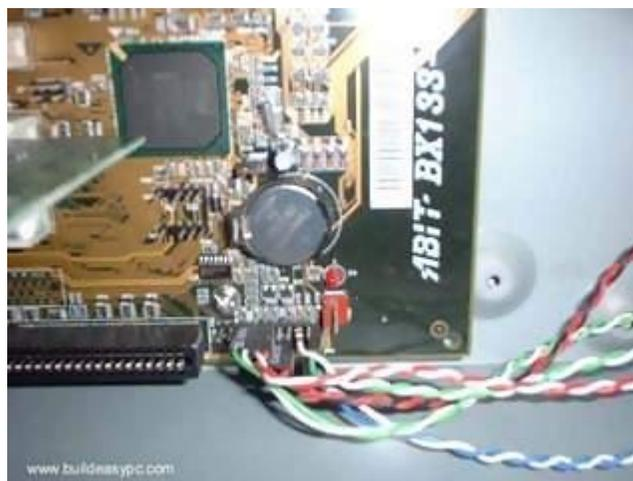
Figure 2 - Switch and LED connectors
