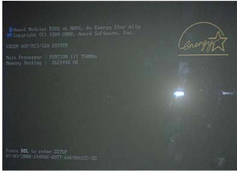
If your motherboard has a plug and play BIOS and is set to automatic device detection by default, then you would see your IDE devices being detected followed by a prompt complaining about missing operating system. If your motherboard does not detect the hardware, then you need to proceed to the BIOS setup screen by pressing DEL or F1 or F2 depending on your motherboard.
