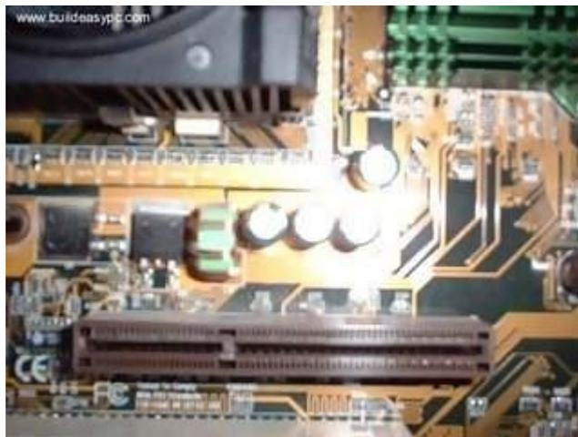
Place your AGP card on top of the slot and gently push it down. The card should firmly sit into position.
