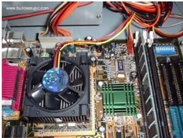
CPU fan has a power connector which needs to be connected to CPU fan power socket on your motherboard as shown on the image above.
