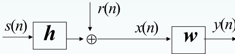
$$W(\omega) = \frac{S_{xd}(\omega)}{S_{xx}(\omega)} = \frac{H(\omega)^*}{|H(\omega)|^2 + \sigma_r^2}$$
