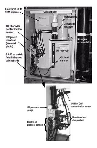
Powerbase offers three self-contained, reliable, HPUs for non governing turbine systems. Each unit is designed to balance cost with product reliability.
