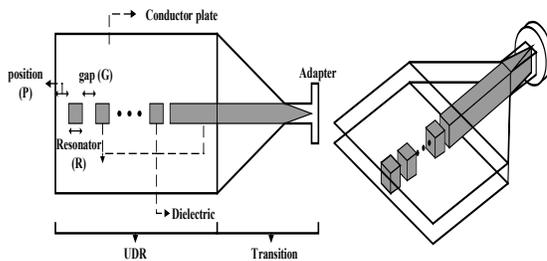
Fig. 1 Structure of a gap-coupled UDR with waveguide to NRD transition
