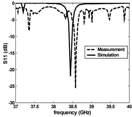
Fig. 5 Simulated and measured  $S_{11}$  of one-pole gap-coupled UDR
