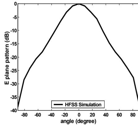
Fig. 8 Simulated E plane pattern of three-pole gap-coupled UDR
