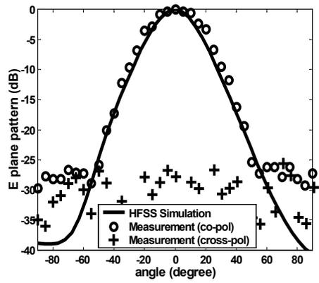
Fig. 7 Simulated and measured E plane patterns of one-pole gap-coupled UDR
