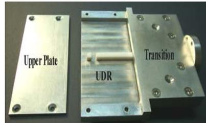
Fig. 2 Photograph of a gap-coupled UDR with transition
