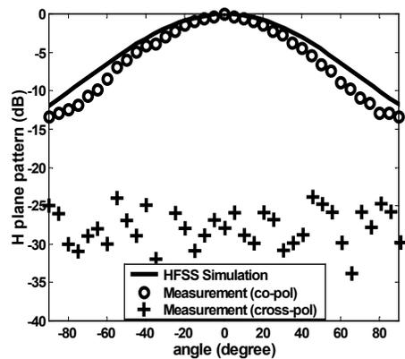
Fig. 9 Simulated and measured H plane patterns of one-pole gap-coupled UDR
