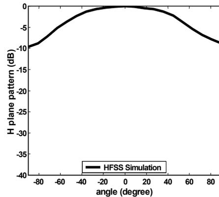
Fig. 10 Simulated H plane pattern of three-pole gap-coupled UDR
