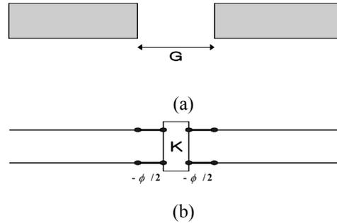
Fig. 4 (a) Dielectric pair separated by gap
