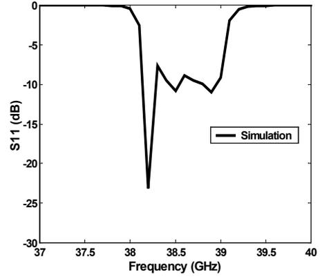
Fig. 6 Simulated  $S_{11}$  of three-pole gap-coupled UDR
