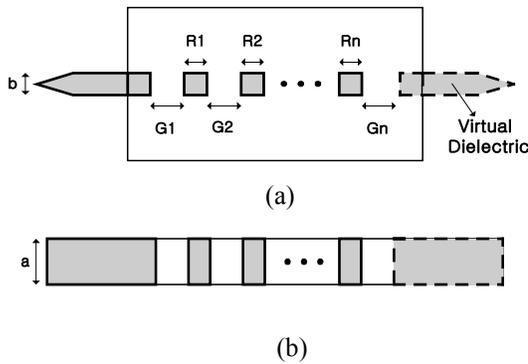
Fig. 3 Schematic diagram of a gap-coupled UDR
