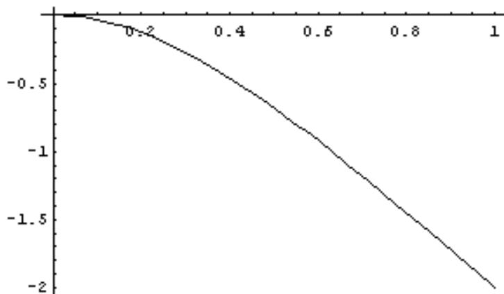
$$\begin{aligned} & C[1] \cos\left[\frac{4.69409x}{L}\right] - C[1] \cosh\left[\frac{4.69409x}{L}\right] - \\ & 1.01847 C[1] \sin\left[\frac{4.69409x}{L}\right] + \\ & 1.01847 C[1] \sinh\left[\frac{4.69409x}{L}\right] \end{aligned}$$
