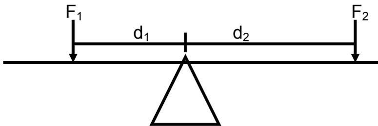
Ex. 13 A crowbar 27 inches long is pivoted 3 inches from the end. If 100-lb of force is applied to the long end, how many pounds of force is there to lift an object at the short end?
