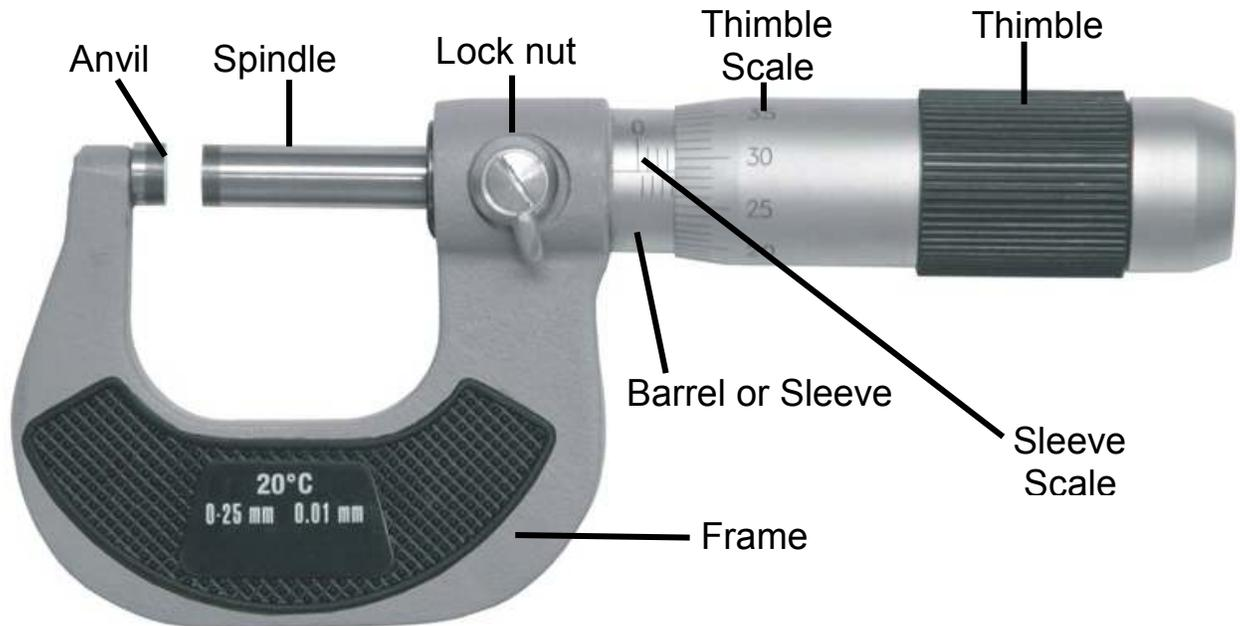
To measure the length of an object, we insert the object in between the end of the spindle and the anvil and turn the thimble until the spindle closes.
