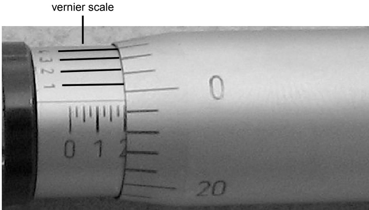
The total distance of the ten vernier scale spaces is equal to the total distance of nine scale spaces of the thimble scale:
