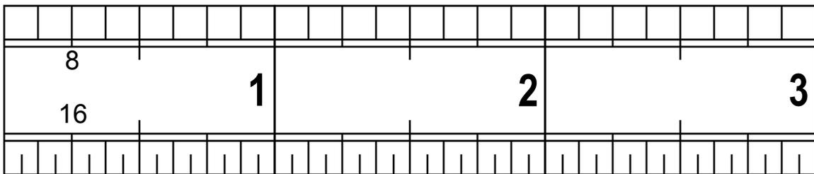
On the top, each inch is split into 8 equal parts. Thus, the 8 indicates the length between two successive marks is one-eighth of an inch. On the bottom, each inch is split into 16 equal parts. Thus, the 16 indicates the length between two successive marks is one-sixteenth of an inch. Let's try reading some measurements:
