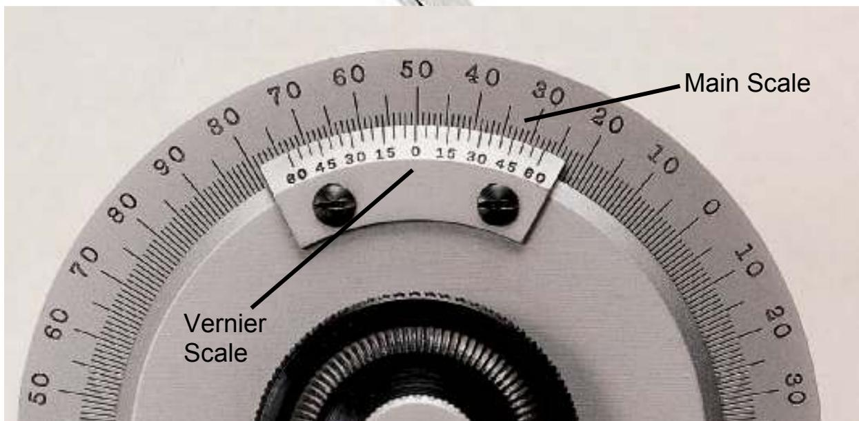
**Reading a Vernier Protractor:**
