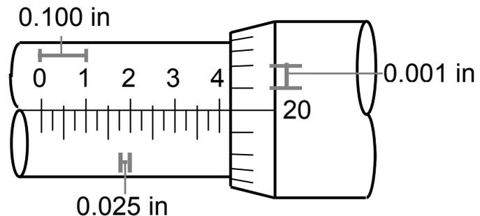
There are four steps we follow when reading an inch-system micrometer.
