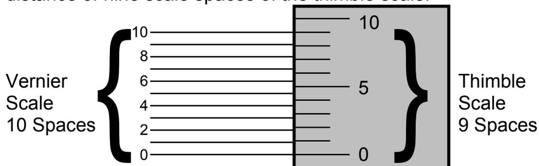
The difference between a space on the vernier scale and a space on the thimble scale is 0.0001 inches. When reading a vernier micrometer, the first three steps are the same as for a regular micrometer. We will then add a fourth step:
