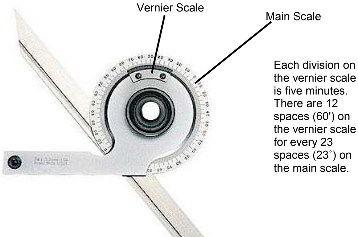
Each division on the vernier scale is five minutes. There are 12 spaces ( $60'$ ) on the vernier scale for every 23 spaces ( $23^\circ$ ) on the main scale.
