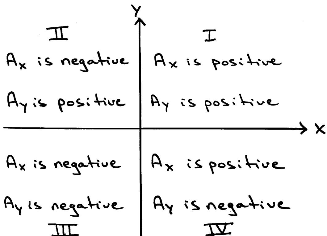
Convention: The positive direction is taken as counterclockwise from the +x axis.
